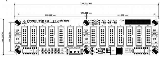
Use 3 mm screws and spacers. U1 can be bolted or soldered.
